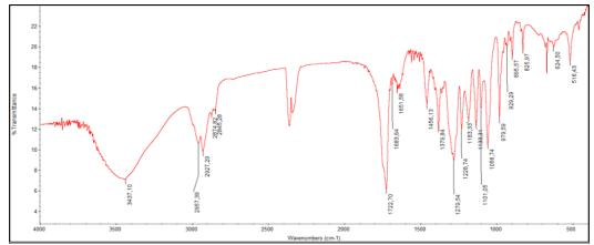
Figure 3. FTIR spectrum of purified PHB from *Brevibacterium* sp. B45 Figure 3. Spektrum FTIR hasil pemurnian PHB dari Brevibacterium sp. B45
