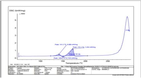
Figure 4. DSC analysis of purified PHB from *Brevibacterium* sp B45 Gambar 4. Analisis DSC hasil pemurnian PHB dari Brevibacterium sp B45
