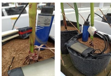
Figure 3. Maize daily water usage measurement with a Sap flow meter
