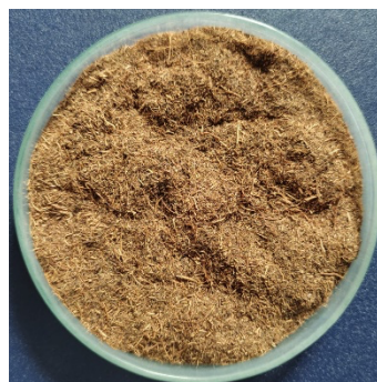
Figure 1. The fibers of oil palm empty fruit bunches (OPEFB) Gambar 1. Serat tandan kosong kelapa sawit (TKKS)
